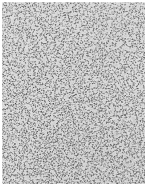
Fig. 9 Image of a dispersion containing 5 g/l ceria in aqueous \text{HNO}_3 at pH 2, obtained through cryo-transmission electron microscopy. The bar represents a length of 200 nm. The ceria particles are the small dark grains, with diameters between 5 and 10 nm. The particles are randomly distributed through the dispersion; this is consistent with SAXS results which show no preferred distances between them at this concentration
